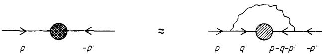
Figure 1. Single phonon exchange contribution to the Dyson equation. Cross hatching denotes the proper self-energy, and diagonal marking the exact propagator of the electron.
